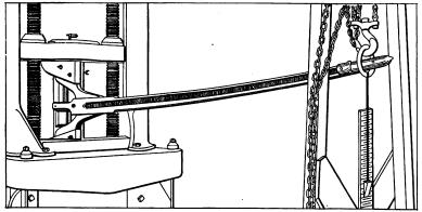
Fig. 59.—Method of testing wagon poles; trussed pole under test.
